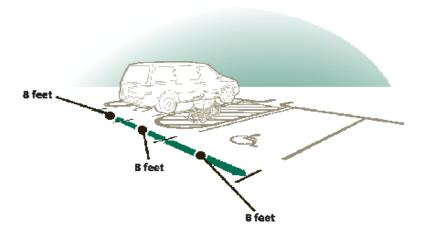
Look for accessible parking. Parking stripes should allow 8 feet for a car/van plus a 96-inch access aisle. The access aisle should be marked with a "No Parking" sign. The accessible spaces should be closest to the accessible entrance, and there should be signs indicating accessible parking. To ensure that only those in need of these parking spaces use them, there should also be an enforcement policy.
